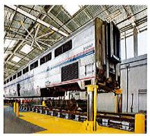
In-Floor Jacks travel parallel and perpendicular to the rail up to 30 feet, making it ideal for repair shops handling various lengths of railcars.
