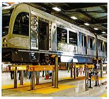
Car Hoist Systems are the safe solution when repairing the railcar underbody and / or side components.
