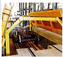
Full Truck Drop Tables allow for the efficient change out of bogey trucks as well as the flexibility to replace single axles & are adaptable to satisfy almost any service requirement or size pit.
