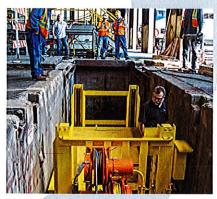
**Single Axle Drop Tables** enable fast and efficient wheel changeouts.
