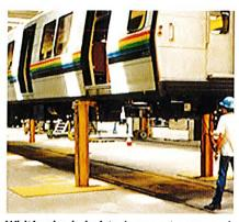
Whiting body hoists / supports are used to facilitate body and truck separation, or to elevate railcars to safe heights and hold them for inspections and repairs under the car.
