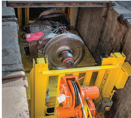
Mechanical and Hydraulic Single Axle Drop Tables enable fast and efficient wheel changeouts.
