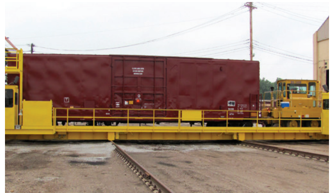
Transfer Tables easily move railcars between parallel tracks for efficient maintenance operation.
