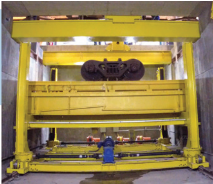
Full Truck Drop Tables facilitate the efficient changeout of locomotive and railcar bogey trucks to minimize downtime and get your equipment back into service.
