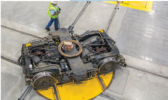
Turntables facilitate transfer of bogey trucks between tracks to improve efficiency and productivity.
