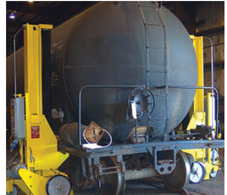
Portable Electric Jacks are available in 35, 50, and 60 Ton capacities to safely service rail cars and locomotives.
