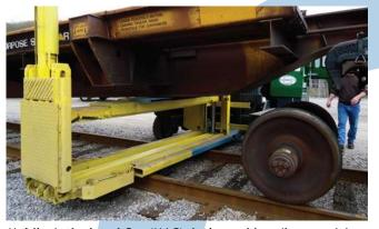
**Mobile Articulated Car (MAC) Jacks** enable railcar servicing anywhere a fork truck can operate.
