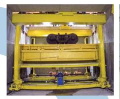
Full Truck Drop Tables facilitate the efficient changeout of locomotive and railcar bogey trucks to minimize downtime and get your equipment back into service.
