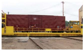
**Transfer Tables** easily move railcars between parallel tracks for efficient maintenance operation.
