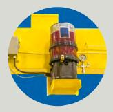
Automatic Jack Screw Lubrication System Dispenses Grease to Lifting Screws During Normal Operation
