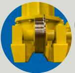
Drop Table Wheel Change Outs are Completed Without Having to Lift the Table Out of the Pit
