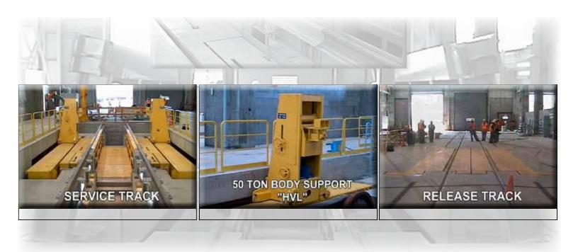
To remove drive wheels or trucks with a Drop Table, the locomotive is located and supported over the table top, where the trucks are disconnected, lowered, transferred laterally and raised to a release track. The trucks can then be moved to a maintenance area where inspection and repair can be performed quickly and efficiently.
