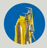
Semi-Automatic or Fully Automatic Table Positioning with Mechanical (shown) or Optical Limit Switches
