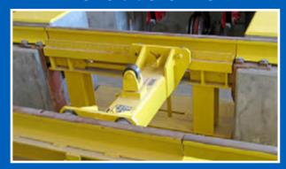
The Traction Motor Dolly provides a controlled method to safely position and support traction motors during the removal and replacement of individual wheel sets.
